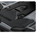
Swim platform with integrated LinQ<sup>™</sup> attachments points An innovative hull that sets the benchmark for rough water handling, stability,
